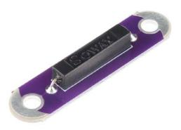
**Description:** The LilyPad Reed Switch is a simple breakout for a reed switch that will make it easy to use in e-textiles circuits in exactly the same manner that you can currently use the LilyPad Button and Switch. In order to make it more durable for wearable use, we've used a different style of reed switch, which is insulated. This means that the same glass switch is encased in black plastic, making it much more difficult to break, but it works in exactly the same manner.
