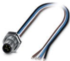
Flush-type connector, Power, 4-position, Plug, Link: M12, T power, Rear mounting, M16 x 1.5, Individual wires, Cable length: 0.5 m
